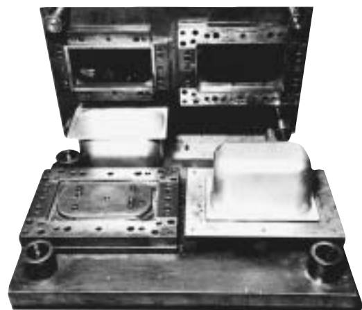
Clipping and edging tool in Uddeholm Arne tool steel to clip and form edge of 0.914 mm (0.036") thick stainless steel container approx. 254 x 152 x 203 mm (10" x 6" x 8").
