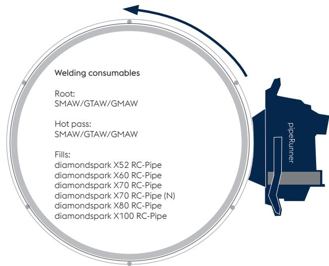
'hybrid' pipeline welding technology for un-alloyed and low-alloyed steel pipelines and pipeworks as proposed by Böehler Welding.
