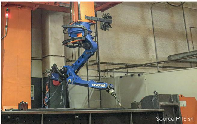
As one can easily guess these applications make large use of robotic welding cells including even complex types (e.g., 2 robots for a large excavator frame) and using sometimes high deposit multi arc MAG processes. Most of the time these installations are equipped with positioners that allow the part to be placed in the most favorable position.
