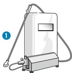
1. Pre-clean, remove oil and grease using Avesta Cleaner 401, and then rinse off with water. Apply the Cleaner with an acid-resistant pump, e.g. Avesta Membrane Pump SP-25.
