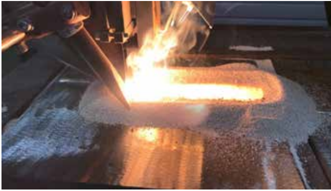
SOU DOTAPE 825H / RECORD 825H HS* - stable cladding process, flat beads and good slag detachability.
