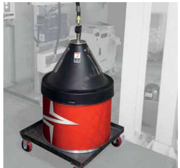
200 kg drum with wire feeding system
