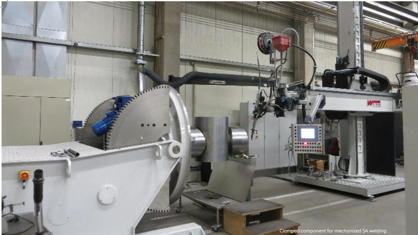
Clamped component for mechanized SA welding
