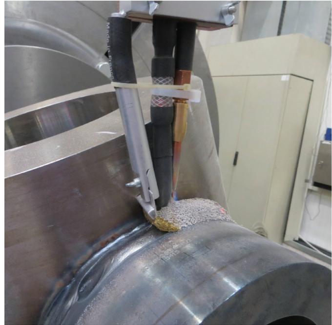
Quality and productivity through automated submerged arc welding
