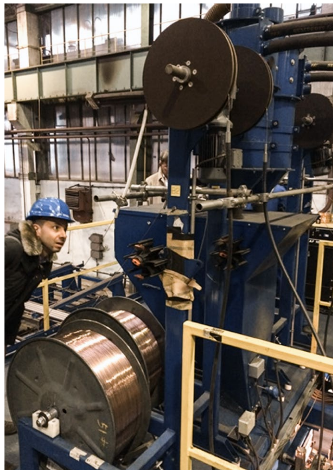
voestalpine Böhler Welding application engineer working on the qualification of Union MV Mo S / UV 305 for fabrication of water wall panels at customer site.
