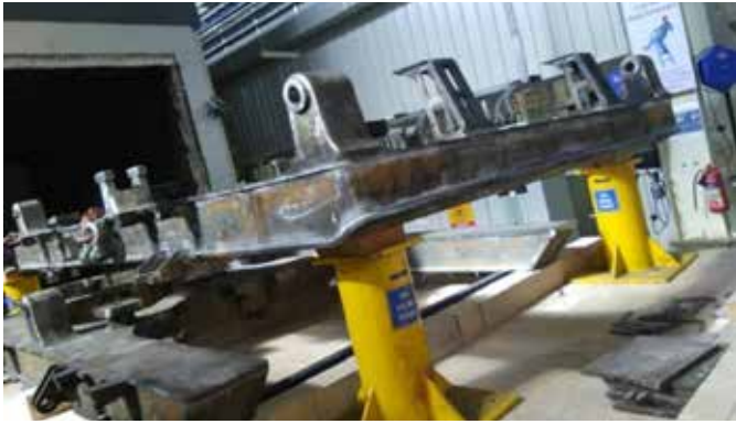
Mock-up frame welded with BÖHLER HL 51 T-MC – a metal-cored wire from the Böhler Welding Diamondspark series. Production of the frames has meanwhile started at General Electric's existing production facility in Pune in the state of Maharashtra to be scaled up when the new factory in Marhowrah becomes operational.
