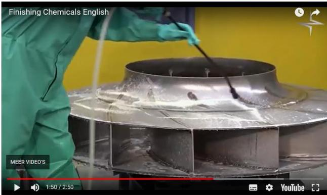
*Spray pickling of an industrial fan in duplex stainless steel. Follow the [link](#) to the video.*
