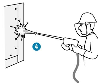
4. Rinse thoroughly with water. There is no need to treat the waste water which is neutral and acid-free. If a complete residue free surface is needed make a final rinse with deionized water.
