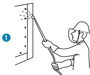
1.1 To avoid smut formation after spray pickling, the passivator shall be applied before rinsing while the surface is still wet, "wet on wet". Leave the fluid to react 30 seconds.
