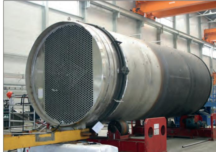
Polysilicon heat exchanger.
