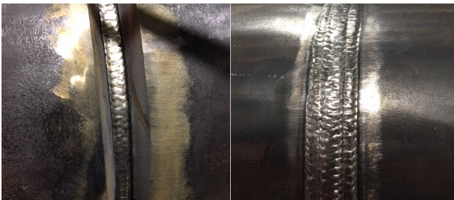
Visual appearance of FOXcore 625-T1 for welding pipes in fixed position. The welds passed x-ray inspection.
