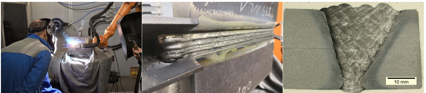
Test of FOXcore 625-T1 for side-wall-in welding of a 30 mm plate with a robotic system to replace SMAW in an LNG application. The weld passed the x-ray inspection.
