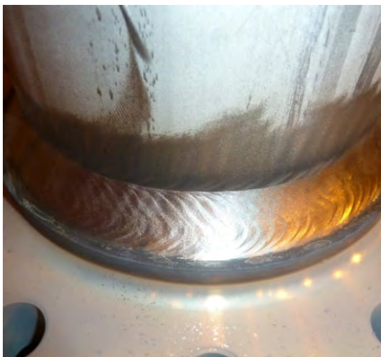
Fillet weld between a tube and flange. Flat position (PB/2F). Base material 1.4307 / 304L. Filler wire Ø 1.2 mm Avesta FCW-2D 308L/MVR. Shielding gas Ar + 18% CO 2 .
