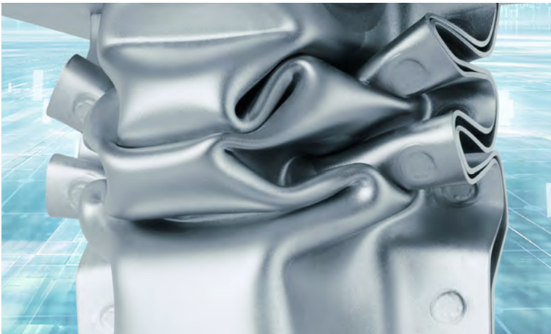
EXCELLENT BUCKLING PROPERTIES OF CR440Y780T-DH
