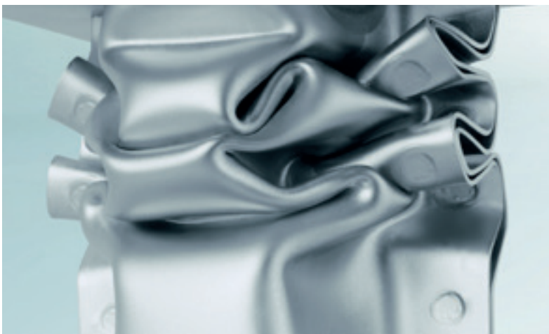
EXCELLENT BUCKLING PROPERTIES OF CR440Y780T-DH
