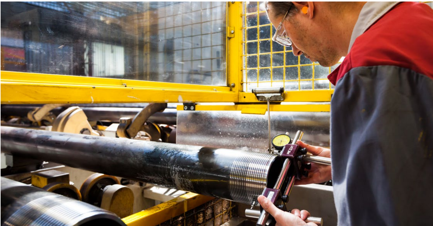
Fig.: Manual thread measurement
