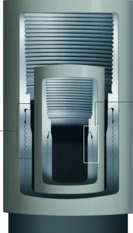
Tubing design 2 % - 4 ½ inches 50% seal taper 7.5° shoulder 2 % - 2 % ": 8 threads per inch 3 ½ " - 4 ½ ": 6 threads per inch 10° stabbing flank 3° load flank
