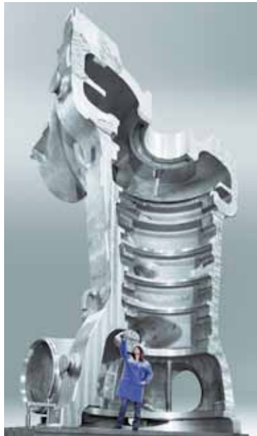
Rough machined MEGA steam turbine
