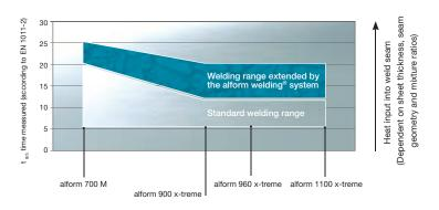
The base material properties were taken into consideration in the design of the filler metals. In combination with tempering-resistant base materials, property profiles occur in the welded joints that allow substantial extension of the welding ranges. The heat input is tendentially higher (longer  $t_{8/5}$  time), increases process reliability (e.g. lower danger of fusion defects) and lowers manufacturing costs because of the increased deposition rate.
