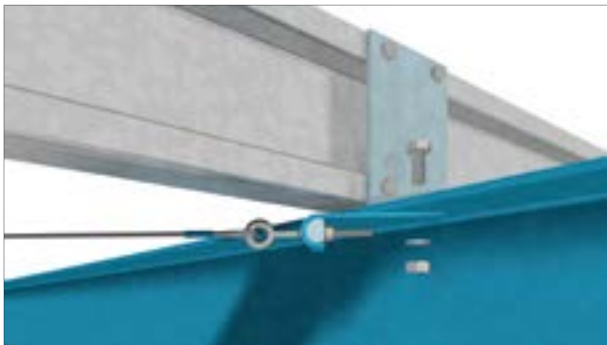
Fitting of diagonal tie to rafter. Using the cleat hole will avoid time consuming drilling of extra holes.*
