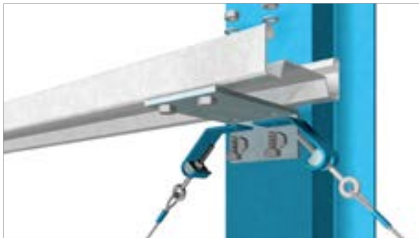
Construction detail of side rail + cleat + diagonal tie wire.
