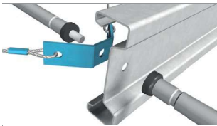
Construction roof purlin + SadeF-Lock® + double diagonal tie wire.
