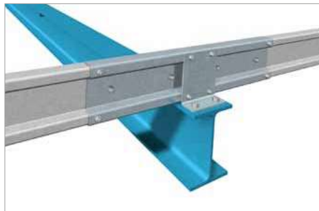
→ Repeat step B and bolt the next sleeved SIGMA to the cleat, using the 2 remaining bolt holes in the cleat.
