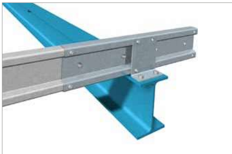
→ Bolting on sleeved SIGMA to cleat, using 2 bolts.
