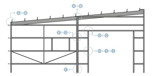
Gable end structures are easy to assemble using cold rollformed sections.
