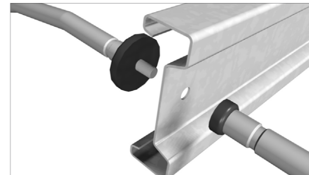
Montagedetail dakgording + noktrekker + SadeF-Lock®
