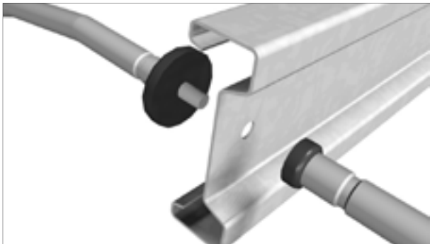
Montagedetail dakgording + noktrekker + Sadeef-Lock®
