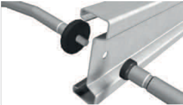
Montagedetail dakgording + noktrekker + Sadef-Lock®
