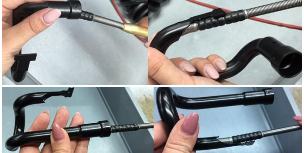
Manual inspection process ensured with endoscope control
