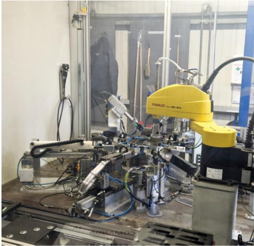
Robot arm pick-up process and transports to 6 control stations
