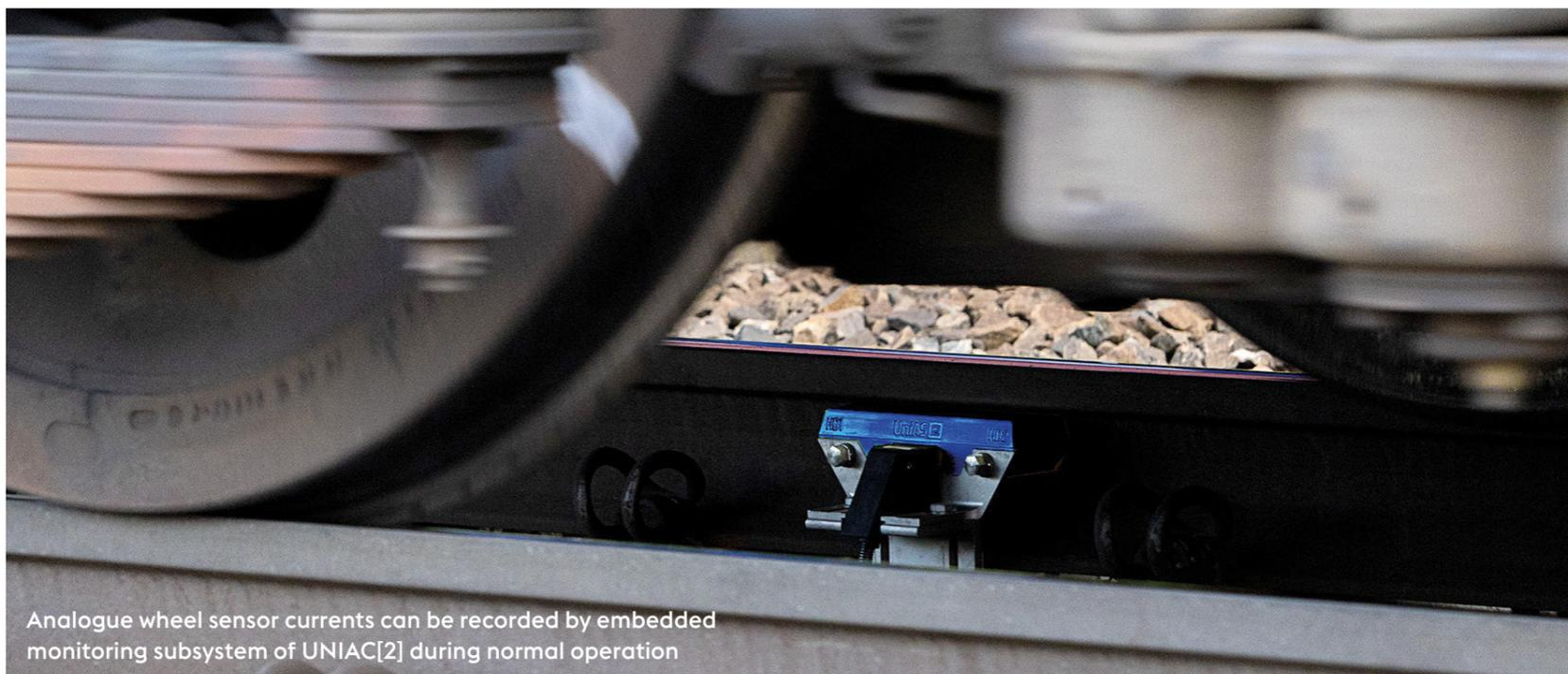
Analogue wheel sensor currents can be recorded by embedded monitoring subsystem of UNIAC[2] during normal operation
