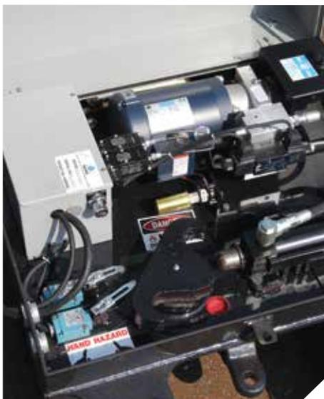
The RACOR<sup>®</sup> Hydraulic Switch Machine is furnished with a hand lever disconnect switch which protects the operator during hand throw operation by automatically disconnecting power to the hydraulic unit. During a trailing movement, the switch points are opened by the wheel flanges, and the throw is completed automatically by the RACOR 22 switch stand, without engaging the hydraulic unit.
