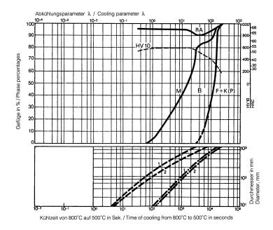
B... Bainite F... Ferrite K... Carbide M... Martensite
