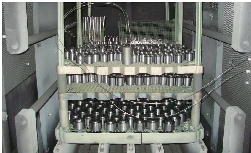
*The use of thermocouples gives an overview of the temperature in different areas during heat treatment. Photo: Böhler Uddeholm Czech Republic*
