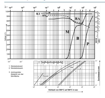
HV10... Vickers Hardness K... Carbide
