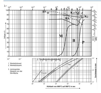
HV10... Vickers Hardness K... Carbide
