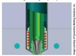
Care should be taken during installation and removal of the nozzle when using a "plunge through" style tip. (Gate inserts can also be used with this tip style.)
