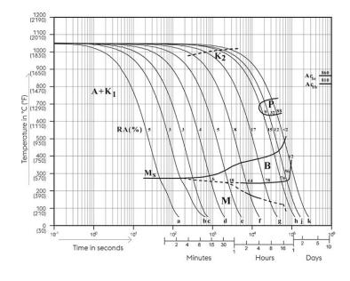
Austenitising temperature:  $1050^{\circ}$ C ( $1922^{\circ}$ F) Holding time: 30 minutes 5...100 phase percentages 0.5...400 cooling parameter, i.e. duration of cooling from 800 -  $500^{\circ}$ C ( $1472-932^{\circ}$ F) in s x  $10^{-2}$
