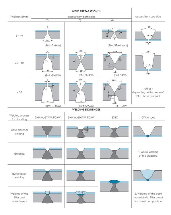
The root gap, the thickness of the root face, the radii and the weld preparation angle depend on the welding processes used. The drawings show examples of dimensions and appropriate processes for welding of the base material. Favourable radii are: r = 8 mm for the base material; r = 4 mm for the clad material and welding with wire electrodes, r = 8 mm with strip electrodes.
