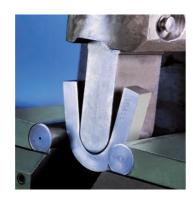
min. 140 MPa acc. to standard (ASTM A264)
