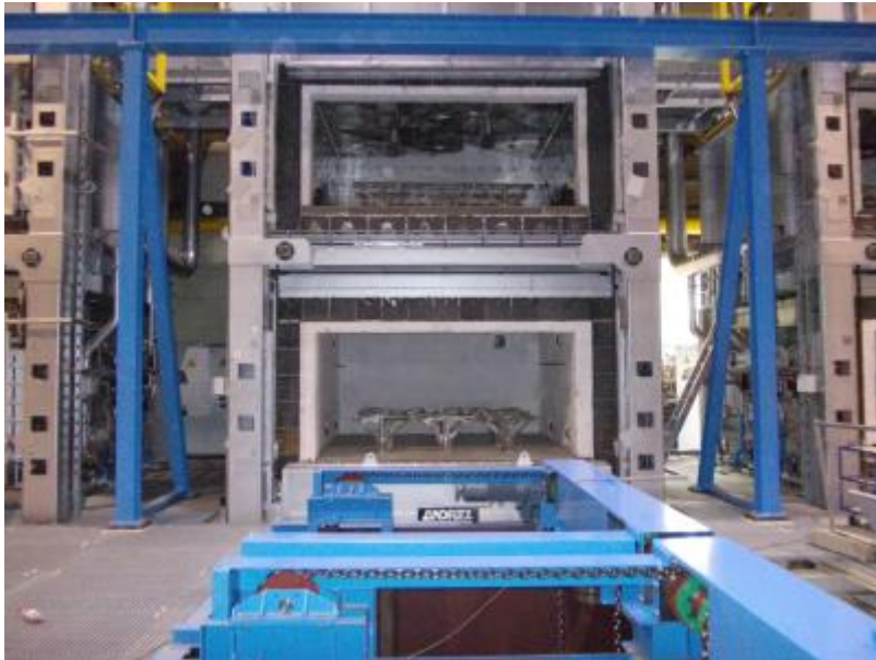
High temperature furnace (HTF, downstairs) and low temperature furnace (LTF, upstairs), quenching bath in front
