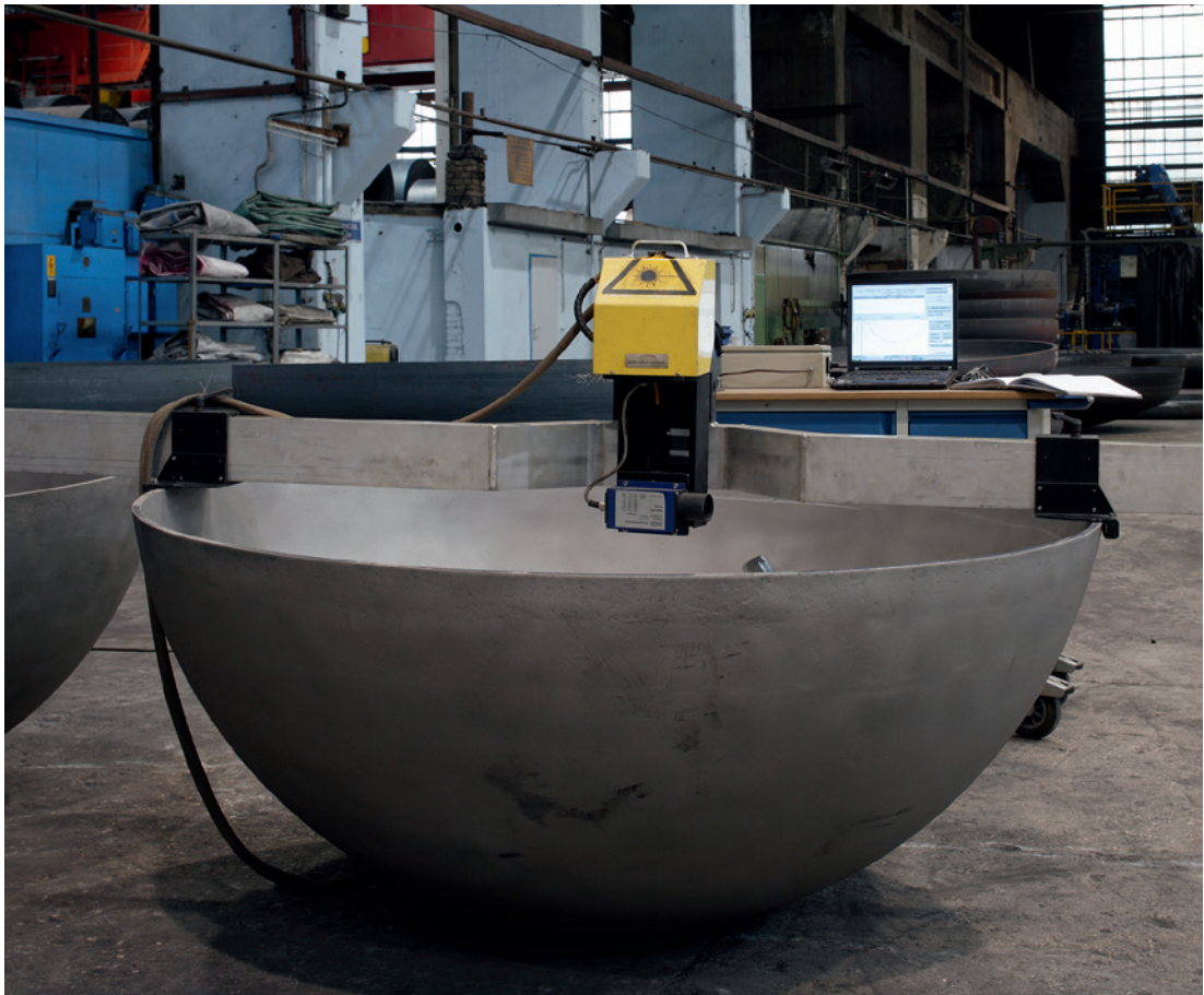
Shape control by automatic laser measurement
