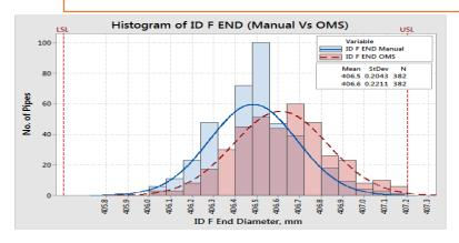
Due to higher precision of OMS compared to manual, standard deviation is more and hence, lower Cpk
