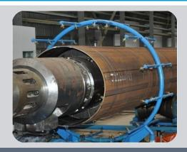
» Mechanical expanders with precisely logic controlled strokes & specially designed tooling to achieve desired mechanical properties (YS/TS) uniformly distributed and precise dimensional tolerance.
