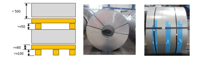
Pack and transport standing coils also in combination with intermediate timbers.
