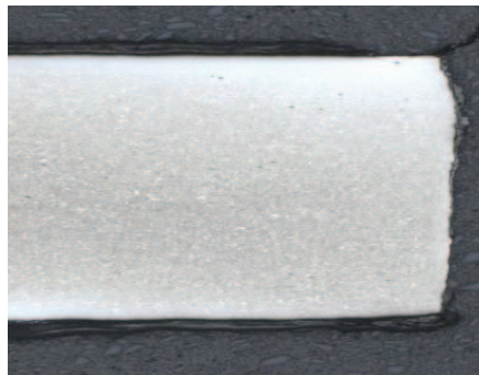
phs-ultraform® 1500 Z140 (hardened) Creepage in transverse microsection after 10 weeks, VDA Test 621-415
