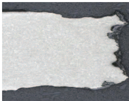
Bright-finished press-hardening steel (22MnB5, hardened) Creepage in transverse microsection after 10 weeks, VDA Test 621-415
