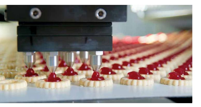
**Portioning units** require high to extremely high corrosion resistance, depending on the foodstuff, and therefore require certification for acidic foodstuffs (pH < 4.5) or testing for aqueous foodstuffs (pH > 4.5).
