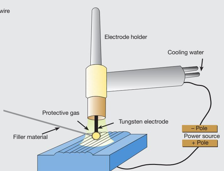
Fig. 2 Gas Tungsten Arc Welding GTAW (TIG)
