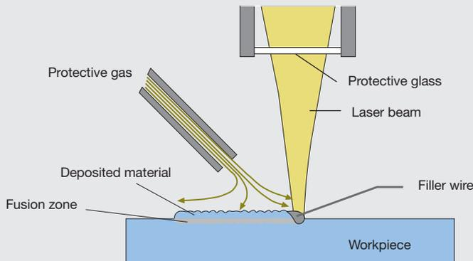
Fig. 3 Laser Welding
