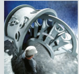
Gas turbine casing
